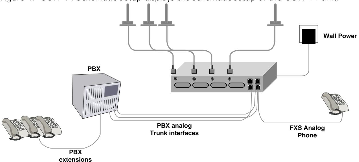
**Figure 4. CGW-T4 Schematic Setup**
