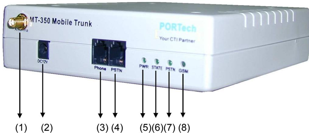
(1) Connecting seat of externally connected antenna.
